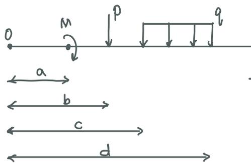
$$\left\{ \begin{aligned} q(x) &= -M \varphi_2(x-a) + P \varphi_1(x-b) + q \varphi_0(x-c) - q \varphi_0(x-d) \\ Q_y(x) &= M \varphi_1(x-a) - P \varphi_0(x-b) - q \varphi_1(x-c) + q \varphi_1(x-d) + 0 \\ M_z(x) &= -M \varphi_0(x-a) + P \varphi_1(x-b) + q \varphi_2(x-c) - q \varphi_2(x-d) + 0 \end{aligned} \right.$$
