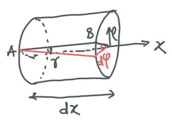
单位长度的扭转角为 \$\theta = \frac{d\varphi}{dx} \rightarrow d\varphi = \theta(x) dx\$
