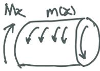
$$M_x + \frac{dM_x}{dx} dx + O(dx^2) \rightarrow \boxed{\frac{dM_x}{dx} + m(x) = 0} \text{ 平衡方程}$$
