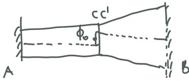
$$\tau_{max} = \left(\frac{TR}{GI_p}\right)_{max} = \frac{2T}{\pi GR^3} \Big|_{max} \rightarrow \text{在AC杆表面处}$$
