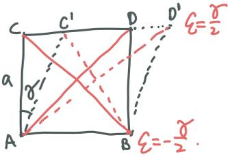
$$AD' = \sqrt{a^2 + a^2(1+\gamma)^2} = \sqrt{2}a \sqrt{1+\gamma + \frac{1}{2}\gamma^2} \approx \sqrt{2}a \left[ 1 + \frac{1}{2}\gamma + O(\gamma^2) \right]$$
