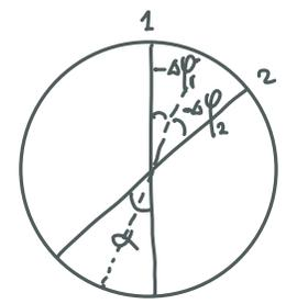
Check: ①  $l_1/G_1 I_{p1} = l_2/G_2 I_{p2} \rightarrow \Delta\varphi_1 = \Delta\varphi_2 = -\frac{\alpha}{2} \checkmark$
