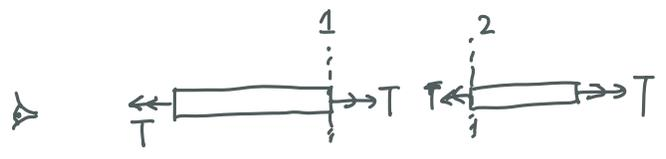
$$\text{物理: } \Delta \varphi_1 = \frac{Tl_1}{G_1 I_{p1}}, \quad \Delta \varphi_2 = \frac{Tl_2}{G_2 I_{p2}}$$
