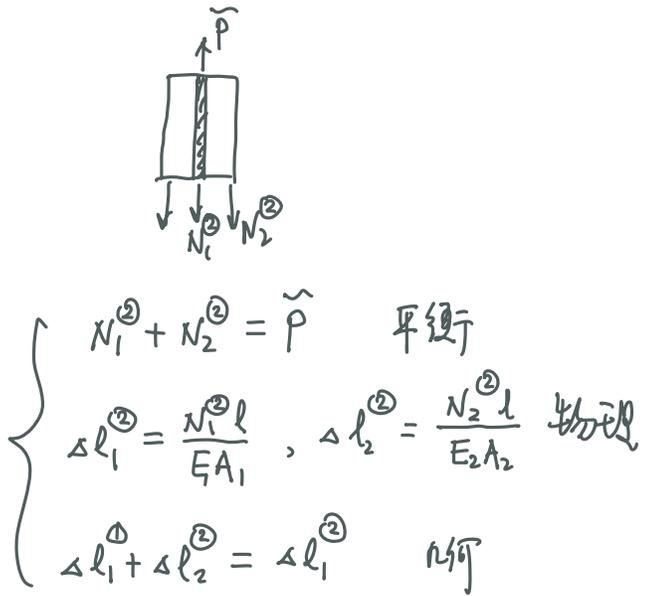
$$\begin{cases} N_1^{(2)} + N_2^{(2)} = \tilde{P} & \text{平衡} \\ \Delta l_1^{(2)} = \frac{N_1^{(2)} l}{EA_1}, \Delta l_2^{(2)} = \frac{N_2^{(2)} l}{E_2 A_2} & \text{物理} \\ \Delta l_1^{(1)} + \Delta l_2^{(2)} = \Delta l_1^{(2)} & \text{几何} \end{cases}$$
