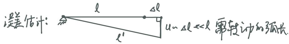
$$l' = \sqrt{(l+\Delta l)^2 + u^2} = (l+\Delta l) \sqrt{1 + \left(\frac{u}{l+\Delta l}\right)^2} = (l+\Delta l) \left[ 1 + \frac{1}{2} \left(\frac{u}{l+\Delta l}\right)^2 + \dots \right] \approx l + \Delta l$$
