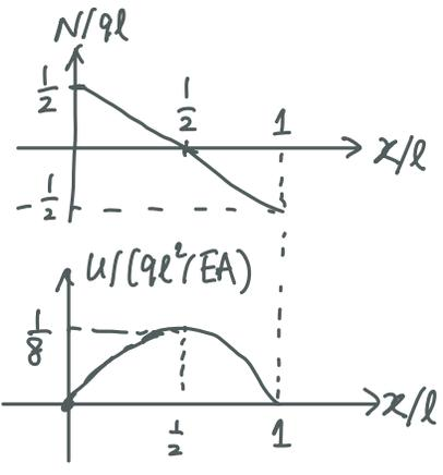
$$\rightarrow N(x) = qL \left( \frac{1}{2} - \frac{x}{l} \right), \quad u(x) = \frac{qL^2}{EA} \left( \frac{1}{2} \frac{x}{l} - \frac{1}{2} \frac{x^2}{l^2} \right)$$
