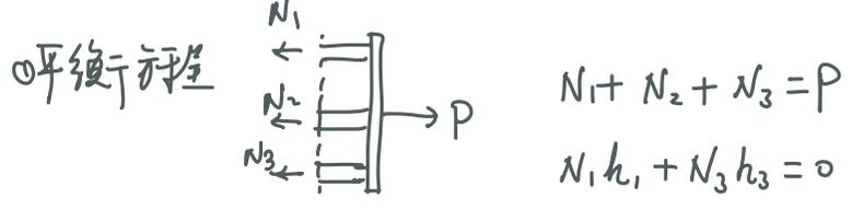
② 物理  $\Delta l_1 = \frac{N_1 l}{E_1 A_1} + \alpha_1 \Delta T$  ,  $\Delta l_2 = \frac{N_2 l}{E_2 A_2} + \alpha_2 \Delta T$  ,  $\Delta l_3 = \frac{N_3 l}{E_3 A_3} + \alpha_3 \Delta T$
