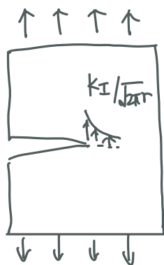
Mode I tensile opening
