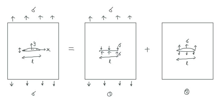
We want to find the potential energy of the system with respect to crack length l. Consider the problem as the superposition of problem O and problem 3
