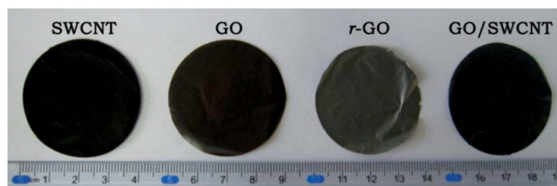
Fig. 2 Digital images of the as-prepared SWCNT, GO, r-GO and GO/SWCNT hybrid films.
